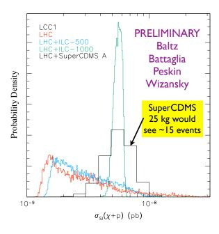
While CDMS-II will continue to advance in the coming year into the low-mass supersymmetric region, SuperCDMS will explore the most favored supersymmetric models in a complementary way to the LHC and a future ILC. As shown in the figure above, there are supersymmetry models (e.g., LCC1 from the Linear Collider Cosmology study) in which SuperCDMS would measure particle physics parameters, such as the WIMP-nucleon cross-section, better than the LHC or even the combined LHC and ILC.
