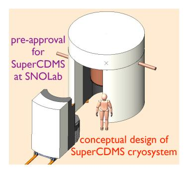
The figure above shows conceptual design work on the SuperCDMS apparatus, including the cryogenic system and the lead and polyethylene shields.
