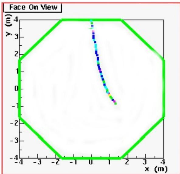
A cosmic ray muon seen in the MINOS detector, entering from the top and headed down. It curves due to the magnetic field and stops before exiting. Each “dot” in this track represents a tiny flash of light in a plastic scintillator strip created when the charged muon passes through. See the [www.soudan.umn.edu](http://www.soudan.umn.edu) website for a live display of current data!
