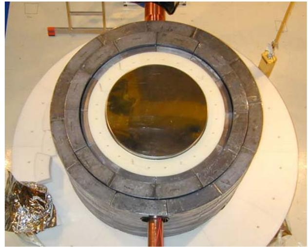
This top view of a partial assembly of CDMS shows the white polyethylene that shields the experiment from neutrons and the gray lead that shields gamma rays. The can lid in the center covers the central cryostat in which the cold detectors are operated.
