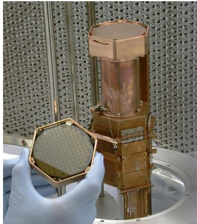
The hexagonal ring holds a single CDMS detector. The square grid on the detector surface shows the patterning of the metallic thermal sensors. In the background is the detector & wiring package forming a “tower”.
