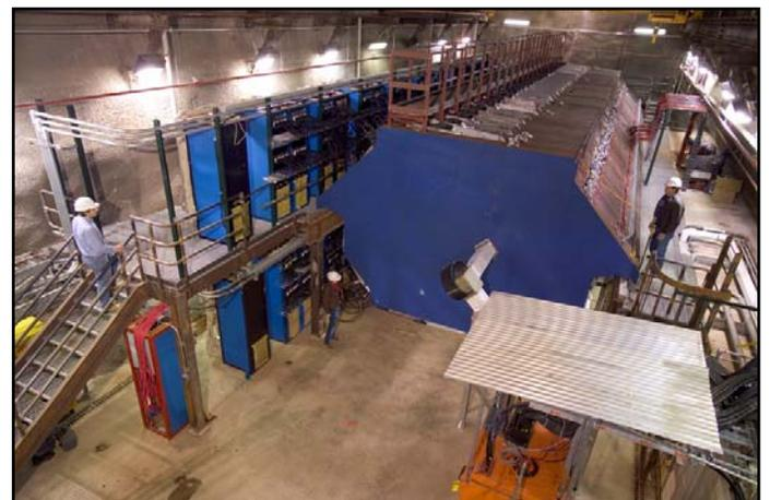
**The MINOS Near Detector, installed at Fermilab.**
